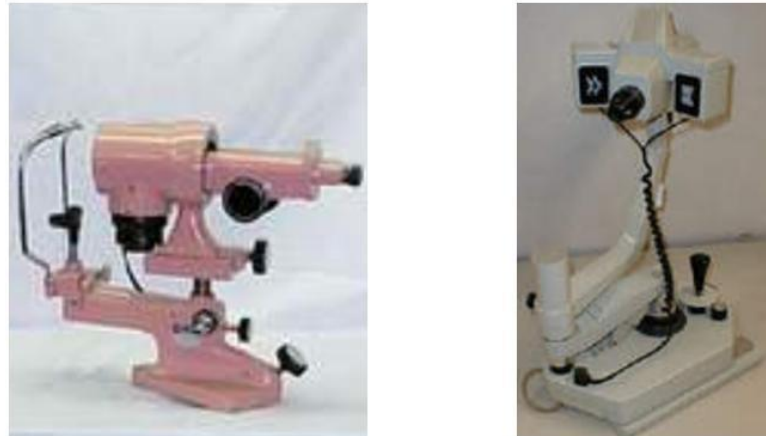
Gambar 2.1. Keratometer (a) Metode Von Helmholtz's (b) Metode Javal-Schiotz
